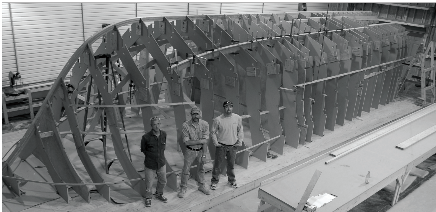
Clay Remick, Dennis Denzin, and Scott Quaintance stand in front of the jigs that will shape the hull of the first custom express to be built by the Ocean Isle-based Island Style Custom Yachts.
